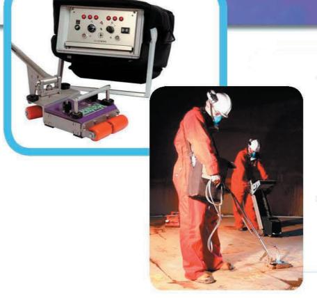
The Handscan system is designed to compliment the MFL 2000 and FloormapVS2i floorscanners. The latest generation of permanent magnets allow localised magnetic saturation of the floor area undertest. As the scanner is moved across the test area signals from the corrosion are detailed by the hall effect sensors.
